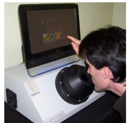
Figure 8. A modern self-administered computerized smell threshold testing device. On a given trial, a pair of stimuli are presented one after the other with a 10-sec interval interspersed. The task of the patient is to indicate which of the two stimuli smells strongest. When misses occur higher concentrations are presented, and when correct responses occur, lower concentrations are presented, in accord with a staircase algorithm. Although programs can also assess odor identification and memory, the main feature of this device is the production of staircase threshold values without the intervention of a tester. Photo courtesy of Sensonics International, Haddon Heights, NJ USA.
